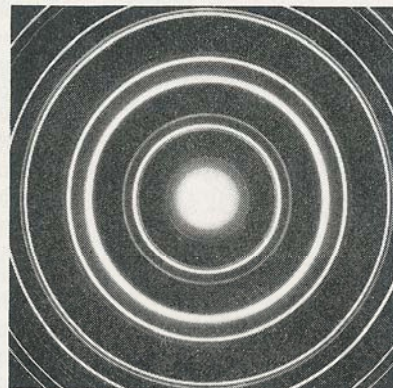
Figure 3-4 Top: The experimental arrangement for Debye-Scherrer diffraction of x rays or electrons by a polycrystalline material. Bottom left: Debye-Scherrer pattern of x-ray diffraction by zirconium oxide crystals. Bottom right: Debye-Scherrer pattern of electron diffraction by gold crystals.
