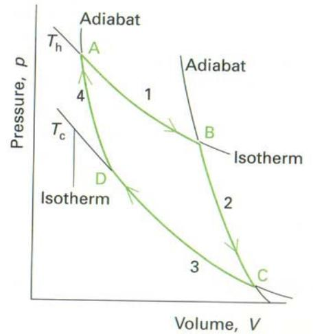
4.5 The basic structure of a Carnot cycle. In step 1, there is isothermal reversible expansion at the temperature  $T_h$ . Step 2 is a reversible adiabatic expansion in which the temperature falls from  $T_h$  to  $T_c$ . In Step 3 there is an isothermal reversible compression at  $T_c$ , and that isothermal step is followed by an adiabatic reversible compression, which restores the system to its initial state.
